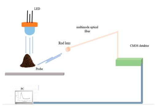
Figure 1. Mobile experimental installation used by fluorescence spectroscopy.
