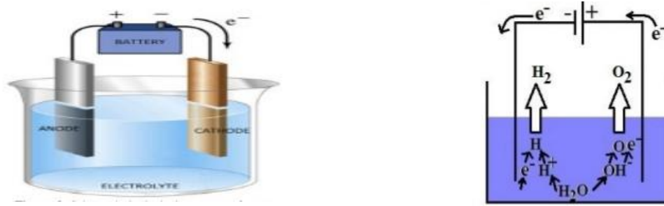
Figure 4. Principal scheme for generating of HHO gas.
