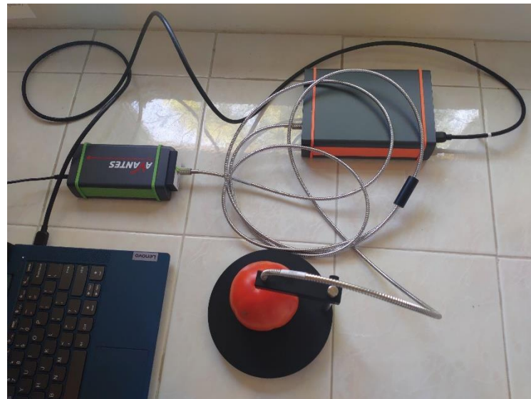
Figure 2. The fluorescence spectroscopy setup for the tomato sample measurements.
