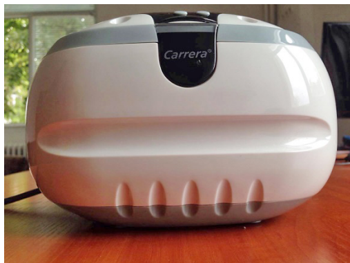
Fig. 1. CARRERA – SINUS ultrasonic bath used to irradiate wheat seeds
