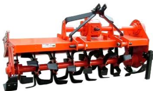
Fig. 75. Rotary tiller with horizontal shaft
