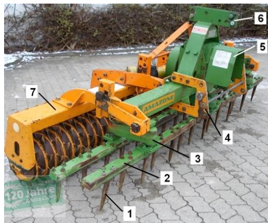
Fig. 83. Power tooth harrow: 1 - tooth; 2 - vibrating beam; 3 - drive arm; 4 - hitching device; 5 – cardan shaft guard; 6 - hitching device; 7 - additional machine (roller)
