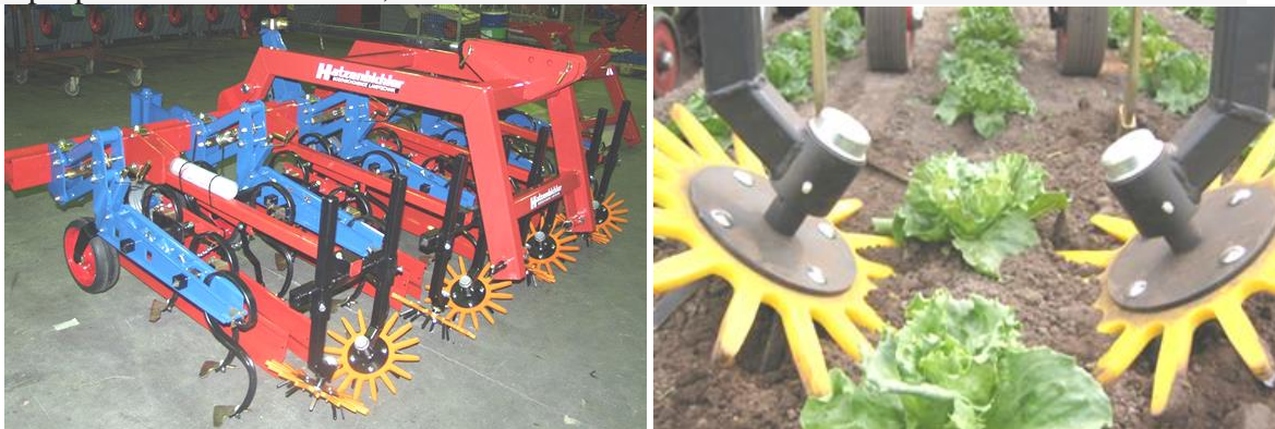
Fig. 70. Cultivator for hoeing with rotating teeth bodies with passive action.
