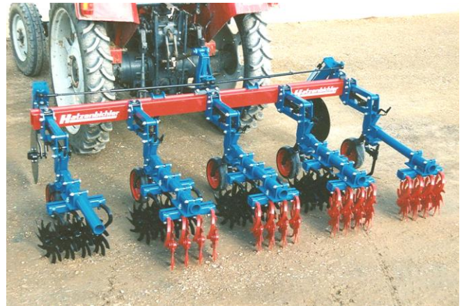
Figure 80. A rear-mounted, row crop rotary cultivator with ground-driven finger wheels
