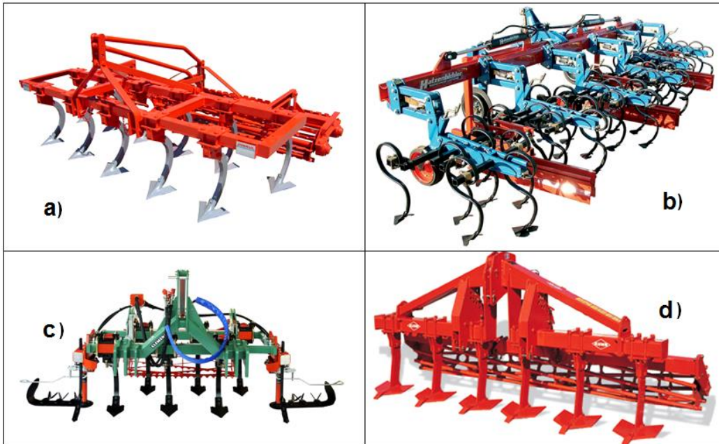
Fig. 64. Types of cultivators: a) field cultivator, b) row crop cultivator, c) cultivator for vineyards and orchards, d) anti-erosion cultivator
