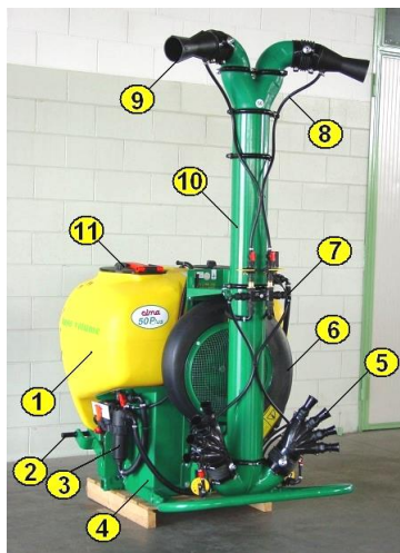
Fig. 21. Tractor pneumatic sprayer: 1 - reservoir; 2 - hitching system; 3 - filter; 4 - frame; 5 - diffusers with nozzles; 6 – centrifugal fan; 7 - solution distributor; 8 - hoses; 9 - diffusers with nozzles; 10 - central air duct; 11 - cover and coarse filter
