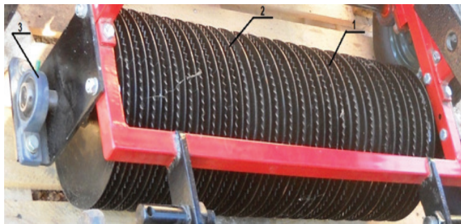
Figure 2. Furrow-forming roller: 1- toothed sector discs, 2- smooth sector discs, 3- bearing body
