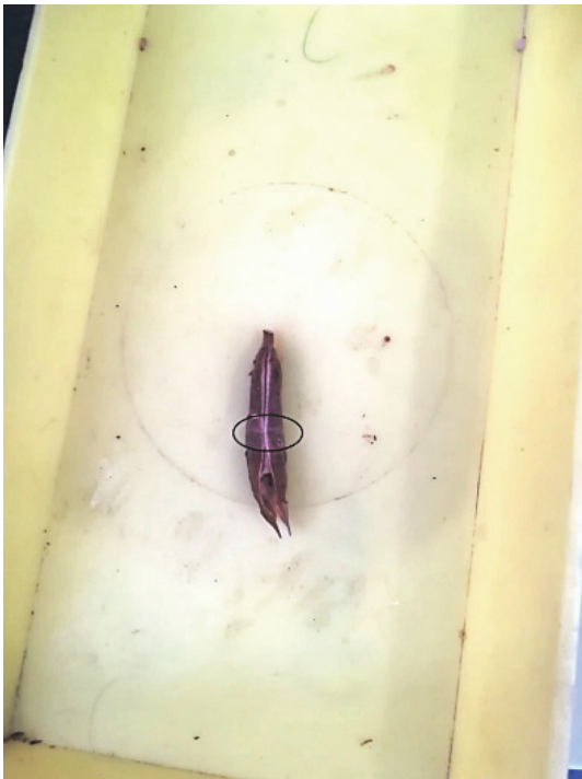
Fig. 9. A capsule damaged by a shock impulse
