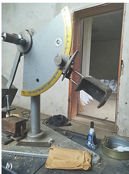
Fig. 3. Pendulum apparatus for testing the susceptibility of sesame capsules for mechanized releasing of seeds: a) at determining indices; b) at determining the proportion of released seeds as a result of shock impulse
